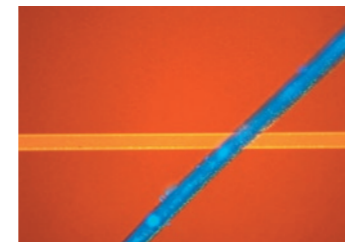
Epi-fluorescence observation of organic substance on wafer
