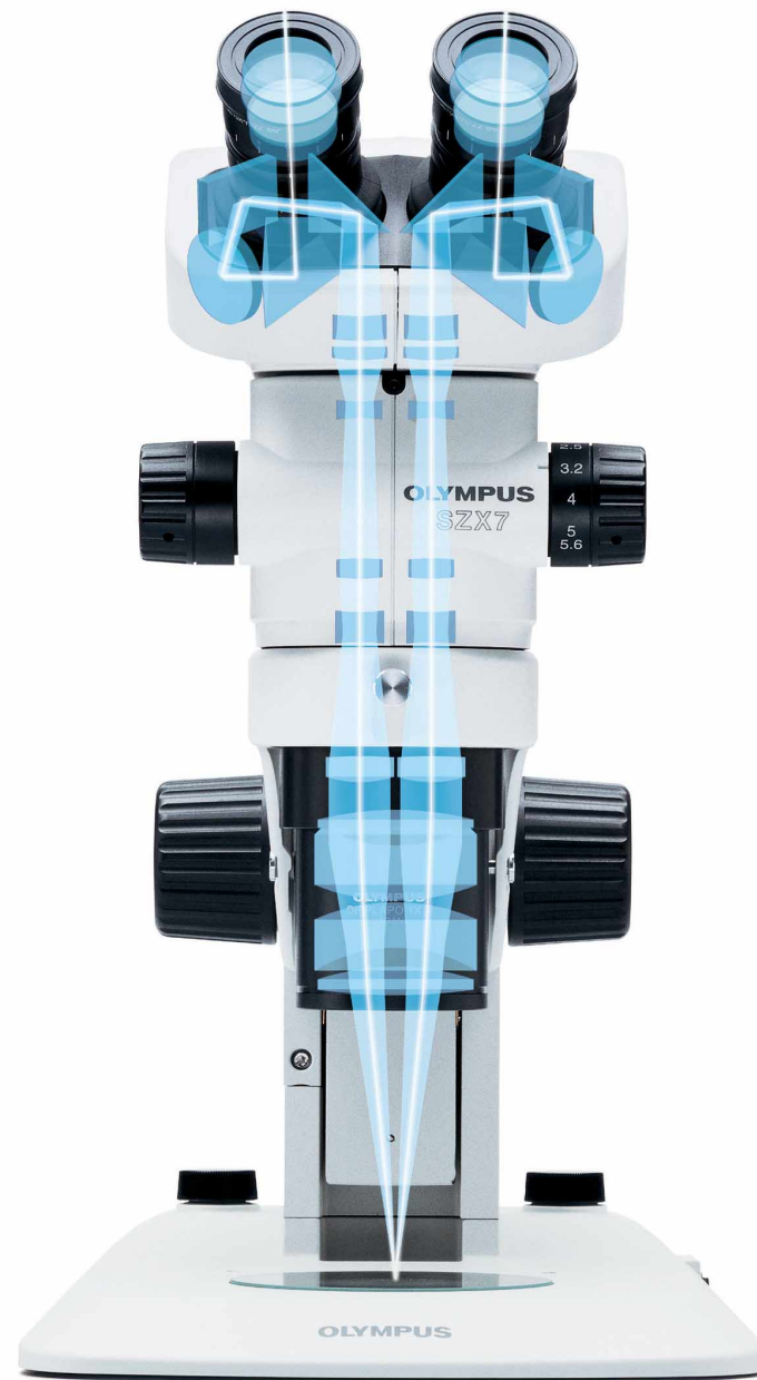
Galilean optics feature two (right/left) independent and parallel zoom optical paths to produce the focal point with one objective lens. The system enables high optical performance as well as functional modularity.
